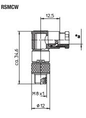
\*a O-Ring \*b Screw joint for cable
