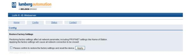
On this web page you can reset the modules to the factory settings. For this purpose, activate the check box and press the button "Apply".
