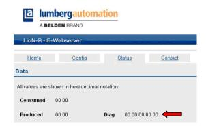
In the data section of the status page up to 5 bytes of diagnostic data are displayed depending on the module. The diagnostic bytes in order from left to right are structured like follows.
